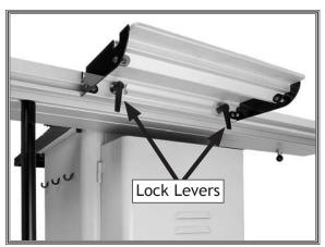
**Figure 12.** Locations of the extension table lock levers.
